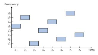
Figure 1. Frequency Hopping Concept.
